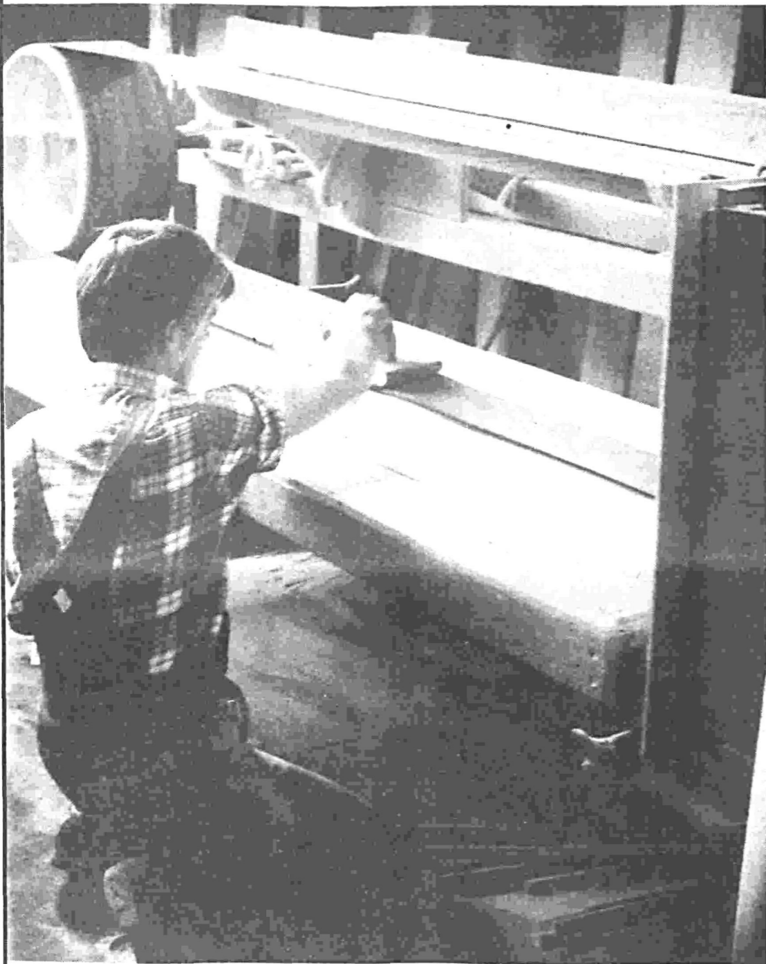
SIMMONS uses a stroke sander to smooth the larger surfaces of the cabinet doors. Bisch's workshop is equipped with many different types of woodworking tools. A table is shown in photo above which Bisch crafted to match an existing set of furniture. He used a drill press for the larger details and handcarved the rest.
