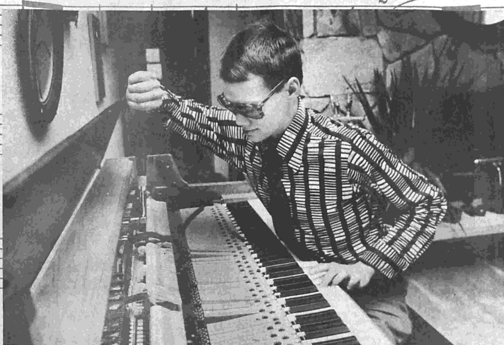
TUNING BEGINS BY muting some of the strings so that each key tone will be harmonized. Here Jerry adjusts the pegs that control those strings. He determines the correct pitch by using a tuning fork.
